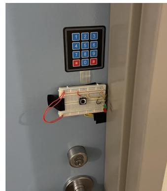
Figure 2: Completed Design Outside of Door
