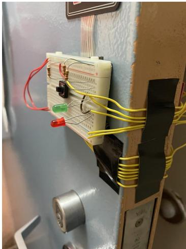
Figure 8: Completed outside circuit showing wires wrapped around the door
