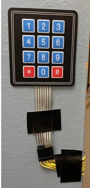
Figure 6: Taping wires down on the outside of the door
