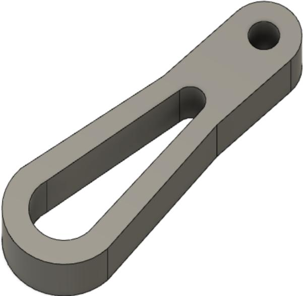
Figure 4: Door Lock Fitting CAD
